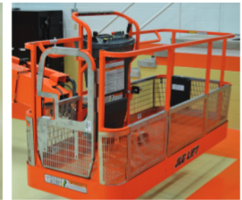
Mesh to Mid Rail
