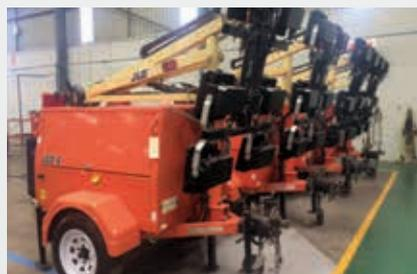
**Refurbished JLG LED 6 head Lighting Towers**
