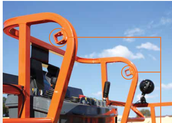
New Platform has two squares welded into the bar (ready for placement of SkyGuard)
