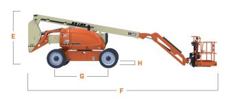
Platform Width 36-in / 0.91-m A. Platform Length B. 96-in / 2.44-m Machine Width 8-ft 2.2-in / 2.49-m D. Tailswing Zero Machine Height 8-ft 5.5-in / 2.58-m E. Machine Length 30-ft / 9.14-m F. Wheelbase G. 8-ft 1.9-in / 2.48-m H. **Ground Clearance** 11.8-in / 29-cm
