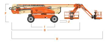
A. Platform Width 36-in / 0.91-m B. Platform Length 96-in / 2.44-m Machine Width - Axles Extended 12-ft 6-in / 3.81-m Machine Width - Axles Retracted D. 8-ft 2-in / 2.49-m E. Tailswing 9-ft 3-in / 2.84-m Machine Height 9-ft 11-in / 3.02-m F. Machine Length - Stowed 37-ft 7-in / 11.45-m G. Machine Length - Overall 47-ft 6-in / 14.48-m Wheelbase I. 12-ft 6-in / 3.81-m Ground Clearance 12-in / 30-cm - Axle 25.5-in / 65-cm - Chassis
