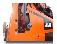
These compact back-up cameras easily mount to the back of the telehandler and provide a wide viewing angle behind the machine. Equipped with infra-red lights, they provide high quality pictures during day or night operation. The images are crisp and clear thanks to the 620 TV lines and the completely waterproof encasing allows them to operate in all weather conditions.
