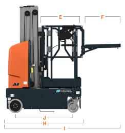
A. Platform Entry Height 18.5-in / 47-cm B. Platform Rail Height 43.8-in / 1.11-m C. Machine Height 78-in / 1.98-m Platform Width 28-in / 71-cm E. Platform Length 29.5-in / 75-cm F. Platform Tray 25-in / 63-cm G. Machine Width 30-in / 76-cm H. Machine Length - Retracted Tray 57.6-in / 1.46-m I. Machine Length - Extended Tray 81-in / 2.06-m J. Wheelbase 41.4-in / 1.05-m K. Ground Clearance 2.5-in / 6.35-cm
