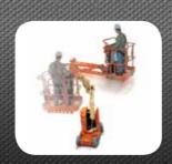
Jib Exclusive JibPLUS® boom option provides 180-degree range of side-to-side movement.
