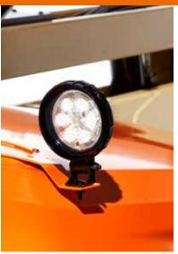
When working in low visibility conditions; use the head and tail lights. These are signaling devices mounted to the front and rear of a boom lift or scissor lift. Head and tail lights help to alert the surrounding environment of the presence of a machine.
