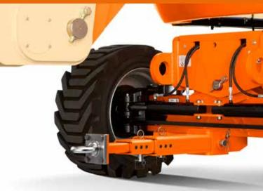
Improve your mobility and rough terrain capability with an oscillating axle. Mounted at the front of the machine, the operator can traverse confidently across uneven terrain with all wheels touching the ground more comfortably and offering more stability.
