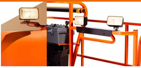
Four 40-watt lights mounted to the chassis; used to illuminate the machine's travel surface. These flood lights will support the platform lights in brightening the work place. It is also part of the Nite Bright® package.
