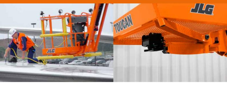
Protect your surroundings and machine with the JLG Soft Touch kit. If the padded framework comes in contact with an adjacent structure, sensors will deactivate platform functions, for increased protection for the surroundings and machine. Ideal for work in delicate environments like aerospace and petrochemical industry.
