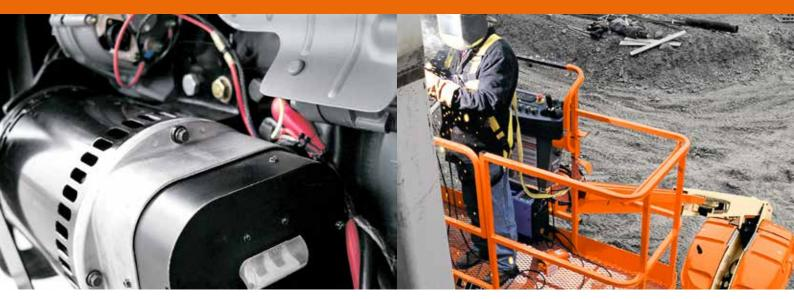
The JLG SkyPower® power to platform system delivers the power you need to conveniently operate other JLG accessories. With the SkyPower® system on your machine, you get a 2500W / 4000W or 7500W generator with a power cable. Easily add and provide power to other JLG accessories, including SkyWelder® in combination with the 7500W generator only.
