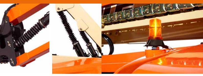
Protect your machine in hostile environments with boom bellows which are mounted on the lift cylinders. The bellows will help protect lift cylinders from dust, sand and debris and offers added protection against salt water damage in coastal regions.
