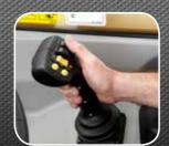
**Single Joystick**The joystick operates boom, attachment and travel functions.
