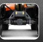
**Heavy Duty**Heavy duty durable axles and permanent 4-wheel-drive with limited slip differential in the front axles.
