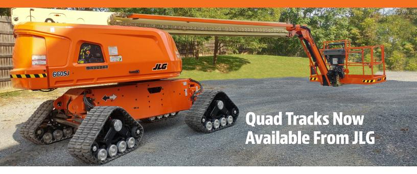
Not all job sites are created equal and each may pose their own challenges and requirements, including the decision of a tracked or wheeled boom lift. **Quad tracks, now available from JLG,** provide the benefit of both continuous tracks and wheels, giving the operator excellent floatation, minimal rutting at job sites, improved traction, superior comfort over obstacles, and best of all no "break over" effect.
