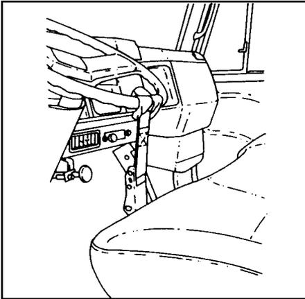
3. It is recommended that the steering wheel of the casualty vehicle be secured by a steering wheel strap for any front or rear tow.
