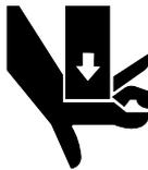
Use only safe practices when maintaining this equipment. Always shut off the engine before reaching into pinch areas.
