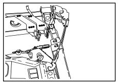
Unhook the wire ropes from their stored position. Moving the wrecker boom with the wire ropes hooked can result in damage to both the wire ropes and the boom.
