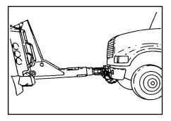
Raise the casualty vehicle into towing position observing the far end for sufficient ground clearance.
