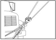
13. Activate the winch free-spool at the controls to re-engage both wrecker boom winches. Slowly take up the slack in the wire ropes. Inspect the hook-up points for slippage before continuing the lift or pull. Control each winch to ensure wire ropes are stressed evenly. As the wire rope is retrieved, be sure it doesn't crisscross on the spool.
