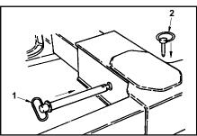
Install the retaining pin (1) from the back side of the crossbar through the grid and crossbar and secure with the pin (2).
