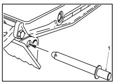
2. Line up holes and insert spade pin (1) and secure with the retaining pin (2).
