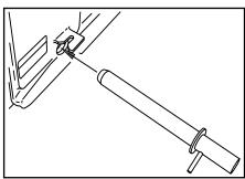
6. Lower the outriggers slightly to gain access to the pinning locations at the upper, inboard ends of the outriggers.
