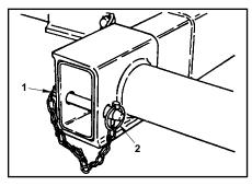
7. Install the retaining pin (1) through the grid and arm weldment and secure with the click pin (2).
