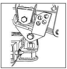
Extend the underlift boom under the casualty vehicle so that the spring lift brackets are in the proper position for lifting. Make sure that the spring lift brackets are against the front part of the spring hanger as shown.
