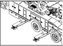
Using the controls, extend the outriggers to the full extended position.
