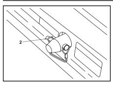
5. Install the pins into the outer sections of the outriggers.
