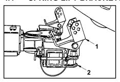
Insert the spring lift brackets (1) into the receivers (2) that you previously installed on the crossbar.
