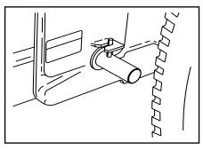
8. Rotate the pin to lock the pin keeper
