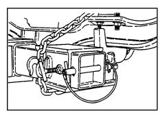
7. After securing the casualty vehicle and before making the final lift, check to be sure that the casualty vehicle's parking brake is released, the transmission is in neutral, and the wheels are straight.
