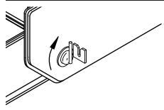
4. Install the pins into the outer sections of the outriggers
