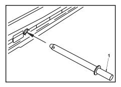
Remove the outrigger pins from the storages compartments. Install the pins (1) into the inner sections of the outrigger and secure with the retaining pins (2). (Three section outriggers only).
