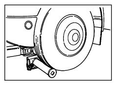
Extend the underlift under the casualty vehicle so that the arm makes contact with the front of the tires.
