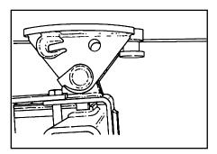
Extend the underlift boom and 5th wheel attachment up to the king pin of the casualty vehicle.
