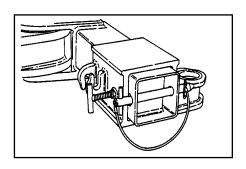
9. Attach the lift receivers to the crossbar by sliding them over the ends of the crossbar. The lift receivers are found in the body tool compartment. Install the retaining pin into the end of the crossbar and secure with the safety pin. Refer to VARIOUS POSITIONS FOR LIFT RECEIVER USE Section 4.2.
