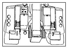
Position the recovery vehicle as close as possible to the casualty vehicle. Set the parking brakes, place the transmission in neutral and chock the wheels.
