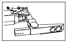
Remove the tire lift grid from the toolbox and slide the tire lift grid onto the crossbar. There are two width positions. The wider width would be used for wide front end lifts for example, and the narrow width would be used for narrower rear end lifts.
