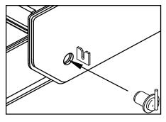
Lower the outriggers slightly to gain access to the pinning locations at the upper, inboard ends of the outriggers.
