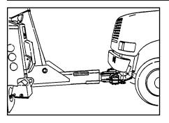
Raise the casualty vehicle into towing position observing the far end for sufficient ground clearance.
