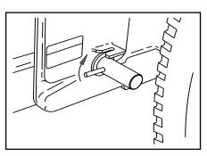
7. Install the pins into the outer sections of the outriggers.
