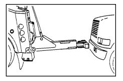
The recovery vehicle's position should be approximately nine (9) feet (3 m) from the casualty vehicle. Reposition the recovery vehicle if necessary.
