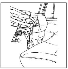
It is recommended that the steering wheel of the casualty vehicle be secured by a steering wheel strap for any front or rear tow.
