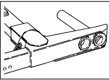
Retract the tube inward to the loading position so that the end of the tube will clear the tires.
