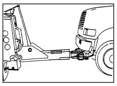
With the casualty vehicle in neutral and the parking brake released, the underlift can be raised, lowered, extended or retracted. All of these movements are hydraulically controlled.
