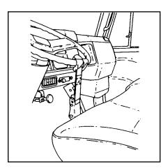
Always secure the steering wheel of the casualty vehicle with a steering wheel strap for any front or rear end tow.
