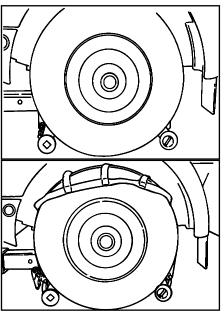
11. Raise the underlift boom to lift the casualty vehicle enough to get the tires off of the ground. Make sure that you are not going to damage any under body components of the casualty vehicle.
