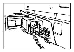
5. Attach hook-up chains to the casualty vehicle. Fasten the chains in the hooks on the end of the adapters and safety wrap the chain around the bottom of the hook as shown. Secure the remaining chain. The use of rubber mats and wood blocks may be required to protect the casualty vehicle.
