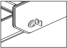
5. Rotate the pin to lock the pin keeper
