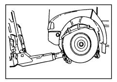
16. Retract the underlift until the casualty vehicle is as close as possible, for the best weight loading, about three (3) to four (4) feet (1 to 2 m) from the back of the recovery vehicle. Leave enough room to maneuver around corners without corner binding or causing contact between the recovery and casualty vehicles.
