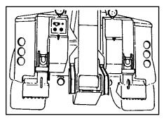
Confirm that the recovery vehicle is positioned properly and rests on firm ground. Properly set the midbody outriggers. The rear outrigger/ spades can be lowered to provide additional support as required.
