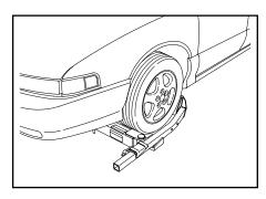
11. Extend the underlift under the vehicle being sure that all under carriage parts are cleared and that the front portion of the grid is in contact with both tires. Lower the grid fully to the ground.
