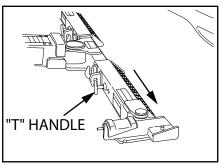
10.Pivot the wheel restraint receivers on the end of the grid arms outward by lifting up on the receiver. Rotate the "Cam" handles on the receivers 180° to the open position for easier placement of the restraint into the receiver.
