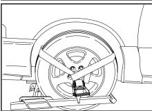
Set the ratchet spool in "free spool" position and pull the webbed strap out and form a loop which will wrap around the tire. Be sure the loop is over a minimum of 1/3 of the tire.
