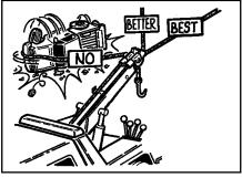
Position and align the truck to obtain as direct a pull as possible. Straight line pulls are the best and most efficient.
