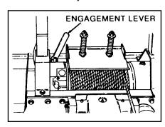
Re-engage the winch and slowly take up the slack in the wire rope/cable. Check all hooks and chains for possible slippage before continuing the lift or pull. As the wire rope/ cable is retrieved, be sure that it doesn't criss-cross on the drum.
