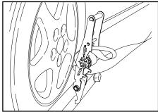
With the vehicle lifted just barely off the ground, attach the strap to the L-Arm. Be sure the hook on the ratchet is securely seated in the L-Arm.
