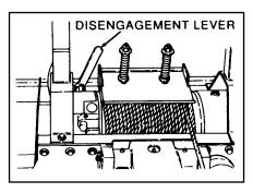
4. Set the boom winch into "free spool" using the disengagement lever. Moving the boom head with the wire rope/cable locked can result in damage to both the wire rope/cable and boom.
