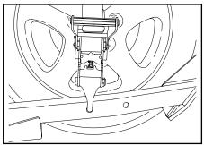
With the vehicle lifted just barely off the ground, attach the strap to the wheel restraints. Be sure the hook on the ratchet is securely seated in the wheel restraint.
