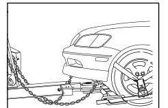
4. Raise the wheel grid to the towing position.
