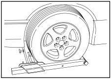
12. Take the L-Arms and slide them into the channels on the side of the grid. Make sure that they are resting snugly against the tires, with the L-Arms in close contact with the tires. Then reset the locking pin by turning the "Cam" handle back to the original position. The tires are now confined front and back. Visually inspect the tire to grid contact before proceeding.
