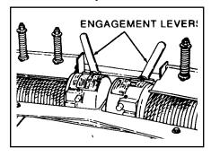
8. Re-engage the winch and slowly take up the slack in the wire rope/cable. Check all hooks and chains for possible slippage before continuing the lift or pull. As the wire rope/ cable is retrieved, be sure that it doesn't criss-cross on the drum.
