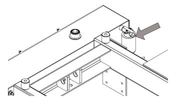
Lube Point(s) - Replaceable Element
