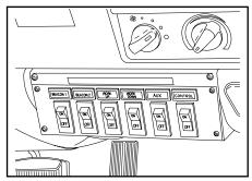
Turn on the safety and work lights. (Switches can be located in the dash panel, in the headliner or in the floor mount.)
