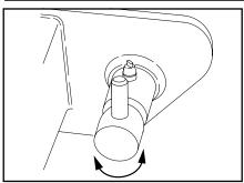
10.Retract the "Cam" handle locking pin on the grid by turning it 180°. It should remain in the open position.
