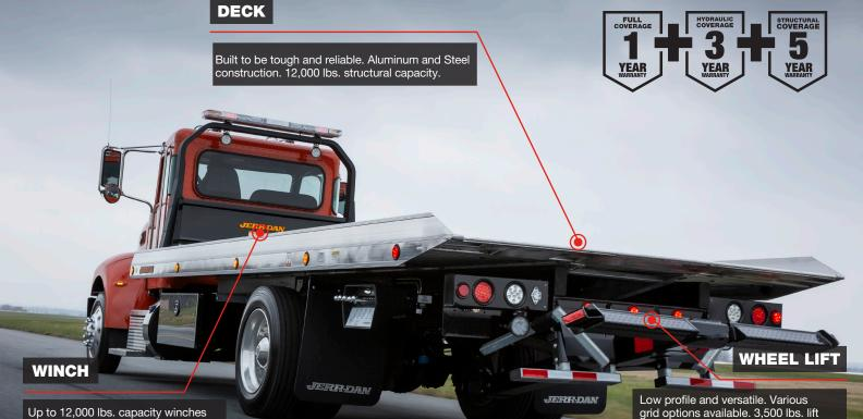
Up to 12,000 lbs. capacity winches for maximum pulling power.
