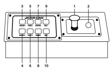
Power Take Off Switch : Engages and disengages the Power Take Off.
