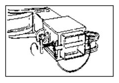
10. Adjust the lift receivers on the crossbar to the desired position and tighten the "T" handles to secure the receivers on the crossbar.
