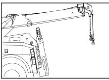
Manually, "free-spool" enough wire rope to make the hook-up being sure that a minimum of five (5) wraps remains on the cable drums.
