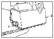
1. Remove the retaining pin (2) and spade pin (1).
