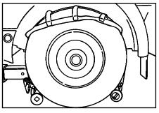
11. Remove the tie-down straps from the toolbox, and attach the hook end of the tie-down strap to the round tube behind the tire. Pull the tie-down strap up and cover the tire and attach the hook on the ratchet end of the tie-down strap to the arm in front of the tire.
