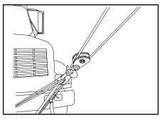
11. The use of snatch blocks and multiple lines will allow you to pull and stabilize the recovery vehicle.
