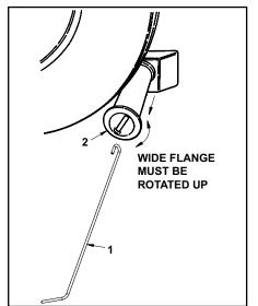
9. Using the pulling tool (1), extend the round tube (2) to capture the back of the tire. After extending the tube beyond the edge of the tire, make sure that the wide flanged edge of the tube is rotated up to prevent the tire from sliding off the end of the tube.
