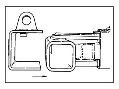
Slide the 5th wheel plate adapter onto the crossbar pivot of the underlift. The 5th wheel adapter plate is stored in the toolbox.
