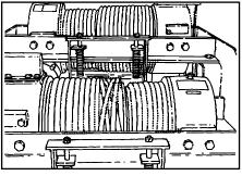
12. Activate the winch free-spool at the controls to re-engage both wrecker boom winches. Slowly take up the slack in the wire ropes. Inspect the hook-up points for slippage before continuing the lift or pull. Control each winch to ensure wire ropes are stressed evenly. As the wire rope is retrieved, be sure it doesn't crisscross on the spool.
