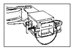
Attach the lift receivers to the crossbar by sliding them over the ends of the crossbar. The lift receivers are found in the body tool compartment. Install the retaining pin into the end of the crossbar and secure with the safety pin. Refer to VARIOUS POSITIONS FOR LIFT RECEIVER USE Section 4.2.
