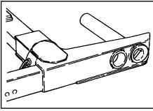
5. Retract the tube inward to the loading position so that the end of the tube will clear the tires.
