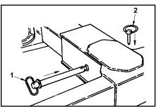
Install the retaining pin (1) from the back side of the crossbar through the grid and crossbar and secure with the pin (2).
