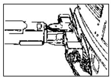
After securing the casualty vehicle and before making the final lift, check to be sure that the casualty vehicle's parking brake is released, the transmission is in neutral, and the wheels are straight.
