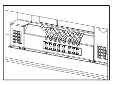
4. Using the winch control levers, unwind some wire rope from the winches to relieve the pressure on the winch free-spool device
