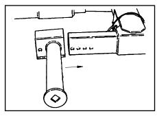
Slide the arm weldment over the end of the grid and adjust to the desired position for loading.
