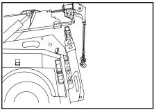
Position the boom head by using the boom up, down, in and out levers as necessary.
