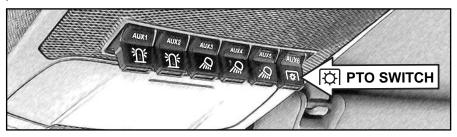
To turn off your PTO, simply turn off the switch marked as the PTO switch. The PTO will disengage, the remote controls will turn off, and any high idle operations will cease.
