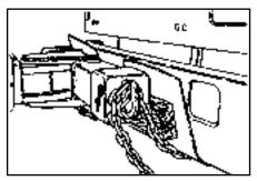
1. Slide the chain hook adapters onto the crossbar.
