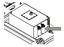
Lube Point(s) – Replaceable Elements Interval – Change every 250 hours or Semi Annually Or as indicated by condition indicator gauges
