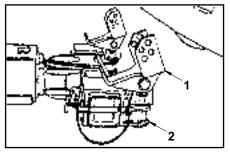
Insert the spring lift brackets (1) into the receivers (2) that you previously installed on the crossbar.
