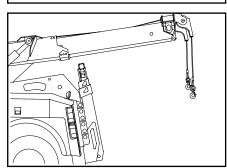
7. Manually, "free-spool" enough wire rope to make the hook-up being sure that a minimum of five (5) wraps remains on the cable drums.
