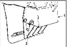
1. Remove the retaining pin (2) and spade pin (1).
