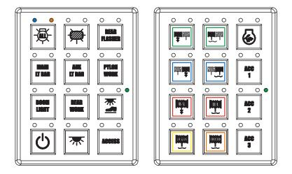
The in-body switch panels are powered by the truck chassis ignition switch. The Green LED will illuminate on the switch panels when the ignition switch is in the on position.
