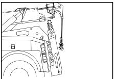
6. Position the boom head by using the boom up, down, in and out levers as necessary.
