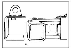
1. Slide the 5th wheel plate adapter onto the crossbar pivot of the underlift. The 5th wheel adapter plate is stored in the toolbox.
