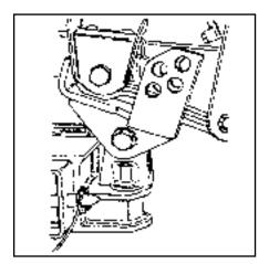
2. Extend the underlift boom under the casualty vehicle so that the spring lift brackets are in the proper position for lifting. Make sure that the spring lift brackets are against the front part of the spring hanger as shown.
