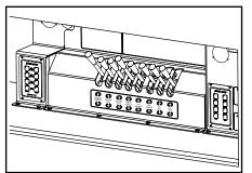
4. Using the winch control levers, unwind some wire rope from the winches to relieve the pressure on the winch free-spool device
