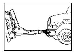
Raise the casualty vehicle into towing position observing the far end for sufficient ground clearance.
