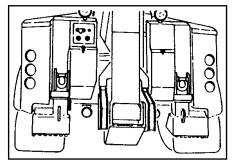
Confirm that the recovery vehicle is positioned properly and rests on firm ground. The rear outrigger/ spades can be lowered to provide additional support as required.
