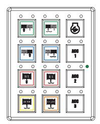
The in-body switch panels are powered by the truck chassis ignition switch. The Green LED will illuminate on the switch panels when the ignition switch is in the on position.
