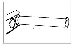
3. Insert the round tube into the desired position in the grid.
