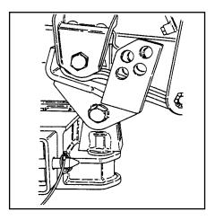
Extend the underlift boom under the casualty vehicle so that the spring lift brackets are in the proper position for lifting. Make sure that the spring lift brackets are against the front part of the spring hanger as shown.
