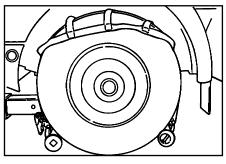
11. Remove the tie-down straps from the toolbox, and attach the hook end of the tie-down strap to the round tube behind the tire. Pull the tie-down strap up and cover the tire and attach the hook on the ratchet end of the tie-down strap to the arm in front of the tire.
