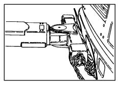
After securing the casualty vehicle and before making the final lift, check to be sure that the casualty vehicle's parking brake is released, the transmission is in neutral, and the wheels are straight.
