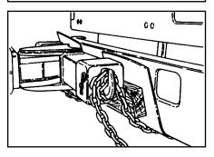
4. Attach hook-up chains to the casualty vehicle. Fasten the chains in the hooks on the end of the adapters and safety wrap the chain around the bottom of the hook as shown. Secure the remaining chain. The use of rubber mats and wood blocks may be required to protect the casualty vehicle.
