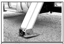
11. If you are on concrete or pavement and can't use the integral spades, pull the spade retaining pin allowing the stabilizer pad to level out flat before completely lowering the stabilizers.
