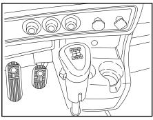
Place the recovery vehicle's transmission gear selector into neutral, set the parking brake and chock rear the wheels.
