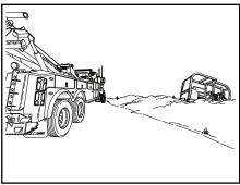
Position the recovery vehicle on firm ground as close as possile to the vehicle that you intend to pull/ recover.
