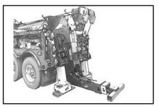
7. Lower the underlift boom to about one (1) in. from the ground.
