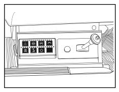
4. Engage the power take-off (PTO) See PTO operator's manual.
