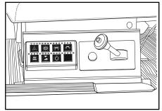
Turn on the emergency lights and auxiliary work lights. Refer to Controls and Indicators Section 3.
