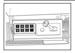
14. Disconnect the power take-off (PTO). Refer to PTO operator's manual. NEVER TRAVEL WITH THE POWER TAKE-OFF CONTROL ENGAGED. This could result in damage to the PTO unit and the recovery vehicle's transmission.
