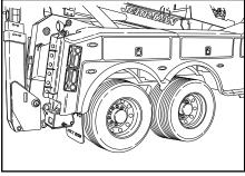
13. Remove the wheel chocks for the recovery vehicle's rear tires.
