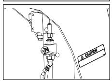
CLOSE the underlift lockout valve located on the tilt/fold cylinder on the back side of the knee boom.
