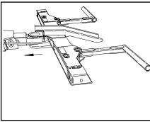
5. Completely retract the wheel grid for loading.
