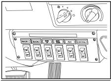
Turn on the safety and work lights. (Switches can be located in the dash panel, in the headliner or in the floor mount.)
