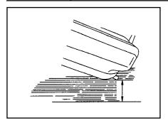
17. Raise the vehicle into the final towing position observing the far end for sufficient ground clearance. It is possible to set the rear of a front lifted vehicle completely onto the ground, causing damage. Take irregular roadsurfaces into consideration. Observe the lift function from the side and away from both vehicles if possible.
