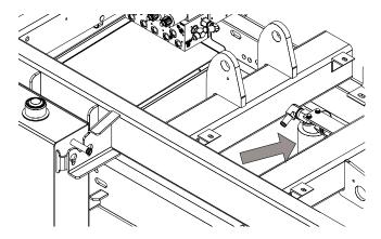
Lube Point(s) - Replaceable Element
