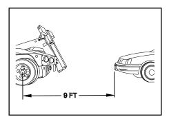
Confirm the truck's position in relation to the vehicle to be towed. Nine (9) feet is recommended. Reposition the MPL-NG if necessary. Be sure the towed vehicle is not in gear or park. Keep the brake set.
