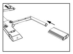
1. Slide the back side of the wheel spacer over the wheel grid arm.
