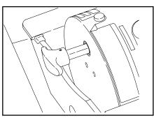
8. Reengage the winch "free-spool" by turning the handle back 90°.
