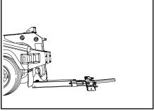
Unfold the under lift boom.
