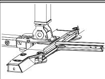
3. Position the gooseneck ball coupler over the ball and lock into place.
