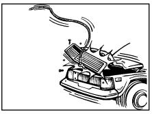
7. Attach the wire rope hook to a chain sling, or bridle and hook securely to the work. Be sure of this hook up; you don't want it breaking loose during the pull. (See the safety sections earlier in this manual). Do not connect to thin or loose body panels or components that could break loose during the winching oper-
