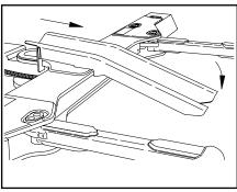
4. Hook the loading ramp onto the wheel grid and engage the rear hooks on the back side of the grid.
