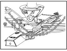
4. Connect the trailer lights and attach safety chains.
