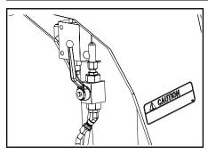
10.OPEN the underlift lockout valve located on the tilt/fold cylinder on the back side of the knee boom.
