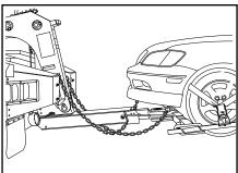
4. Raise the wheel grid to the towing position.
