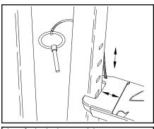
7. Adjust the upper and lower tire stops so that they will contact and restrain the front tire when loaded.
