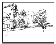
14. Raise the underlift boom to the desired towing height.
