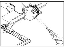
Unwind some wire rope and run the wire rope hook through the recovery sheave.
