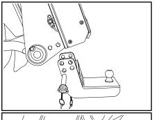
1. Remove the towball hitch attachment from the toolbox.
