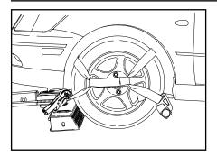
5. Raise the wheel grid to the towing position.
