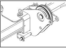
6. Remove the wire rope retaining pin from the grid recovery sheave.
