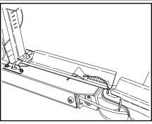
6. Attach the lower trough and vertical stop into the mounting bracket at the front of the boom with the pin and retaining pin.
