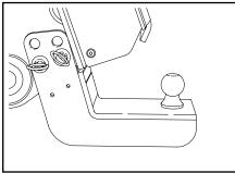
4. Install the desired towball to the towball hitch.
