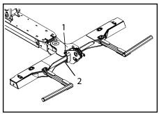
Install the grid recovery sheave onto the back side of the grid crossbar and secure with the pins (1) and hair pins (2).
