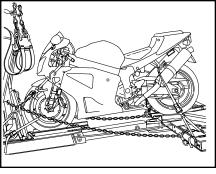
17.Use the wheel lift safety chains to prevent the wheel grid from pivoting during travel. Loop the end of the safety chain around the grid and secure with the grab hook. Remove the slack in the chain and secure the chain in the keyslot of the chain box.
