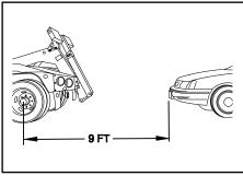
Position the truck within 9 ft. of the subject vehicle and as close to the direction of the pull as possible.
