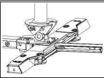
3. Position the gooseneck king pin coupler over the fifth wheel plate and lock into place
