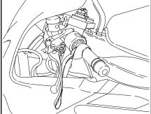
15. Tie the front of the motorcycle to the rear of the wrecker body. Attach the lasso style straps to each of the handle bars.
