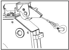
5. Disengage the winch "free-spool" by pulling out on the "T" handle and turning the handle 90°. The handle should remain in the "free-spool" position. This allows the wire rope to be pulled directly off the drum to the work.
