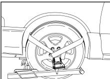
Set the ratchet spool in "free spool" position and pull the webbed strap out and form a loop which will wrap around the tire. Be sure the loop is over a minimum of 1/3 of the tire.
