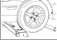
Next, lower the underlift using the underlift down function on the hand controller. The underlift level stop assist system will stop the underlift travel at a preset position about 1-1/2" to 2" from the ground.
