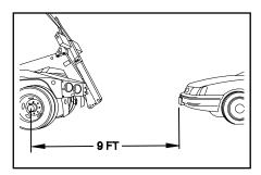
Confirm the truck's position in relation to the vehicle to be towed. Nine (9) feet is recommended. Reposition the MPL-NG if necessary. Be sure the towed vehicle is not in gear or park. Keep the brake set.
