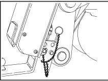
3. Secure the hitch pins with the lynch pins.
