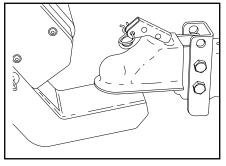
5. Position the ball coupler over the ball and lock into place.
