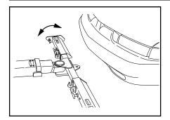
Next, lower the underlift using the underlift down function on the hand controller and swing the cross bar parallel to the tires. The underlift level stop assist system will stop the underlift travel at a preset position about 1-1/2" to 2" from the ground.
