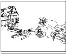
9. Push the motorcycle up the ramp until the front wheel is resting in and against the tire stops in the front brackets.
