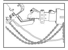
6. Connect the trailer lights and attach safety chains.
