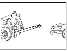
Using the hand controller, unfold the underlift using the tilt down function. The underlift level stop assist system will stop the underlift travel at a preset position.
