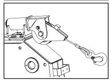
10. With the wire rope tight, slowly wind it in, observing both the work and the drum. Inspect the hook-up points for slippage before continuing the lift or pull. Be sure the wire rope strands do not cross wrap or criss-cross on the drum. Observe the path the work must travel for snags or obstructions which could stall the movement and overload the wire rope.
