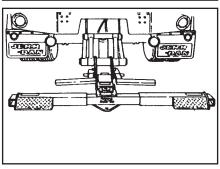
3. Set the brakes on your Jerr-Dan unit. If the pull will be a heavy one you may also use the controls to set the grid boom down on the ground giving the truck more traction and resistance to slippage. The use of scotch blocks is also recommended.
