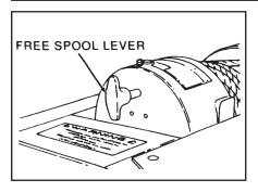
4. Release the free spooling lever on the winch by pulling and turning the handle 90°. Never pull this while the wire rope/ cable is under load! This allows the wire rope/cable to be pulled directly off the drum to the work.
