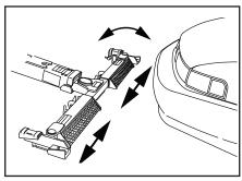
9. Set the grid width as required for the vehicle to be towed. To set the grid width, loosen the "T" handles on the front of the grid arms and pull out. Be sure both grids are as close to the center of the boom as possible, and wide enough to allow the L-Arms to slide into their channels. Tighten the "T" handles to secure the grids
