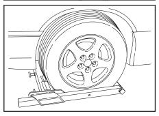
12.Take the L-Arms and slide them into the channels on the side of the grid. Make sure that they are resting snugly against the tires, with the L-Arms in close contact with the tires. Then reset the locking pin by turning the "Cam" handle back to the original position. The tires are now confined front and back. Visually inspect the tire to grid contact before proceeding.
