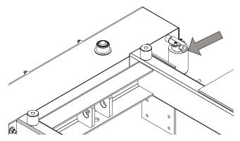
Lube Point(s) - Replaceable Element
