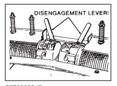
4. Set the boom winch into "free spool" using the disengagement lever. Moving the boom head with the wire rope/cable locked can result in damage to both the wire rope/cable and boom.
