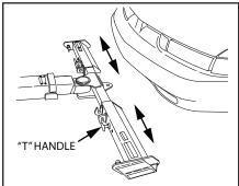
9. Set the grid width as required for the vehicle to be towed. To set the grid width, loosen the "T" handles on the front of the grid arms and pull out. Be sure both grids are as close to the center of the boom as possible, and wide enough to allow the L-Arms to slide into their channels. Tighten the "T" handles to secure the grids
