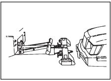
Position the truck within 3 to 4 ft. of the subject vehicle and as close to the direction of the pull as possible.
