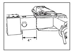
22. Power retract the grid boom until the towed vehicle is about 3 to 4 feet from the back of the truck. Leave enough room to maneuver around corners without corner binding causing contact between the two (2) vehicles. Be sure that the boom is extended at least 4" to ensure unobstructed crossbar pivoting.
