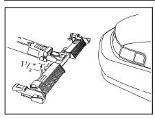
8. Lower the lift arm to about 1-1/2" from the ground and swing the cross bar parallel to the tires..
