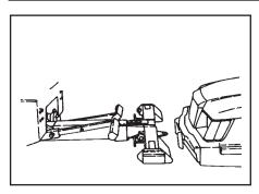
Confirm the truck's position in relation to the vehicle to be towed. Three (3) to four (4)) feet is recommended. Reposition the HPL if necessary. Be sure the towed vehicle is not in gear or park. Keep the brake set.
