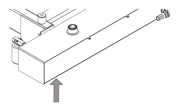
Lube Point(s) - Hydraulic Reservoir Magnetic Plug Interval - Clean every 50 hours or monthly
