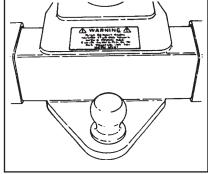
damage the surface if the wheel grid is moved. The grid must be fully retracted against the stop, thus restraining the cross bar from pivoting. Periodically check to assure that the grid has not drifted away from the stop causing hazardous stopping or backing up. Do not tow without attaching safety chains.
