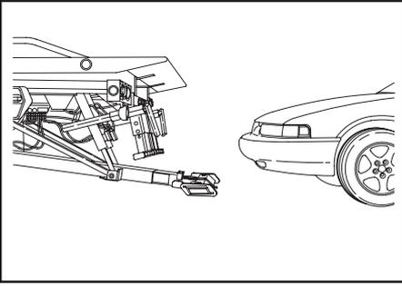
7. Lower the Tow Option Raise/Lower Control handle to lower the wheel lift to about 1-1/2" from the ground. Make sure that it will clear the underside of the vehicle when the wheel lift boom is extended.
