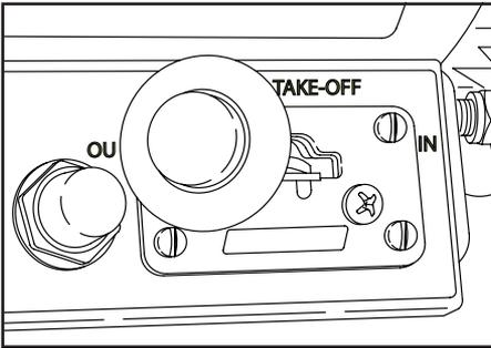
19. Disconnect the power take-off (PTO). Refer to PTO operator's manual.
