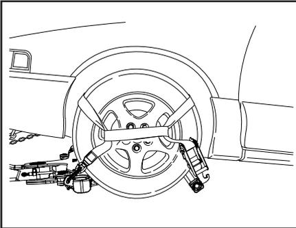
5. Raise the wheel grid to the towing position.
