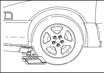
8. Raise the Tow Option Extend/Retract Control handle to extend the wheel lift under the vehicle. Make sure all undercarriage parts are cleared and that the ramp portion of the of grid is in contact with the tires.
