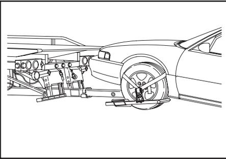
15. Lower the Tow Option Extend/Retract Control handle to retract the wheel lift until the vehicle is about 3 to 4 feet from the back of the truck. Leave enough room to maneuver around corners without corner binding or causing contact between the (2) vehicles. Be sure that the boom is extended adequately to ensure unobstructed crossbar pivoting.
