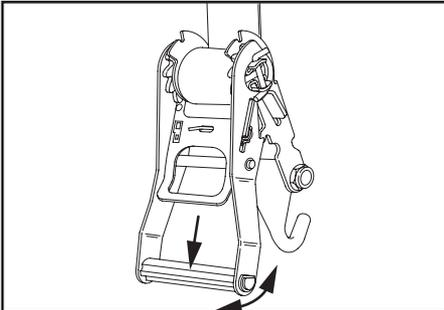
1. First set the spool into “free spool”. This is done by pulling the lock bar out and swinging the handle upward until it rests in the free spool notch and then simply pulling out the amount of strap required to fit over the tire.
