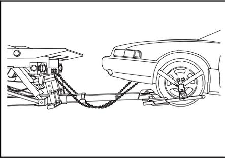
16. Be sure to maintain sufficient clearances with the bottom of the vehicle.
