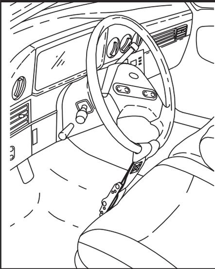
12. Place the vehicle's transmission in Neutral and release the parking brake. Make sure that the wheels are straight and install a steering wheel strap. It is recommended that the steering wheel be secured by a steering wheel strap for any tow.
