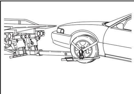
13. Raise the Tow Option Raise/Lower Control handle to raise the wheel lift until the vehicle is in the final towing position.
