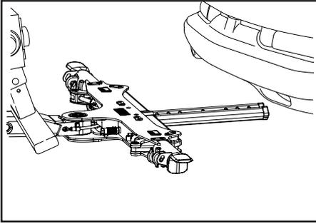
1. Unfold and open the grid arms for loading.
