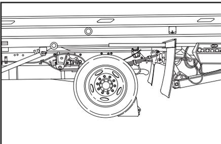
6. Block the carrier's rear tires with wheel chocks to prevent accidental carrier movement. Check the area around the carrier and the equipment to be loaded for obstructions or hazards.
