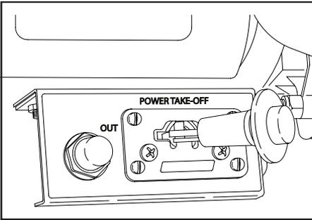
4. Engage the power take-off (PTO). Refer to PTO operator's manual.
