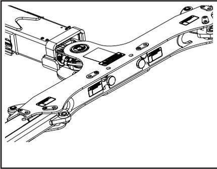
1. Remove the reese hitch adapter bracket from the toolbox.
