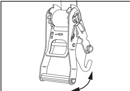
2. Now pull on the lock bar and move it downward until it engages the ratchet teeth on the take-up spool. By pushing and pulling the handle up and down, the strap will be wound onto the spool.
