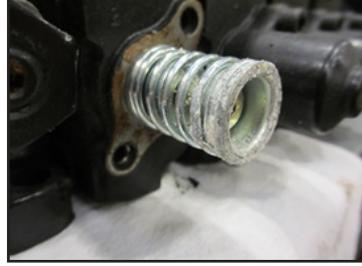
Apply an approved lubricant to protect those components and reduce the likelihood of further build up. Apply the lubricant generously to spring cap end hardware parts (spring seat, spool end, spring and the inside of the cap itself) to insure complete exposure of all part surfaces to the lubricant. This will ensure optimum operation of your valve sections over the life your equipment.
