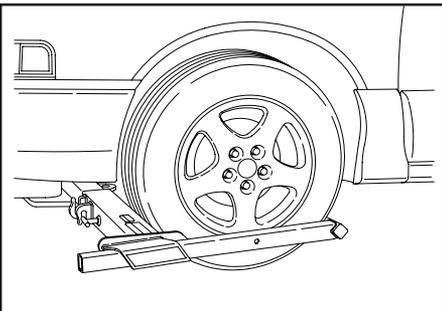
10. Raise the Tow Option Raise/Lower Control handle to raise the wheel lift until the vehicle's tires have cleared the ground.
