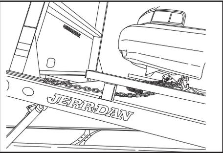
2. Insert the other end of the chain into the keyslot in the deck. Adjust the chain so that it is as tight as possible.
