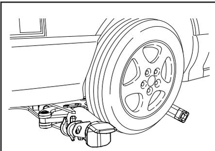
3. Visually inspect the tire to grid contact before proceeding.
