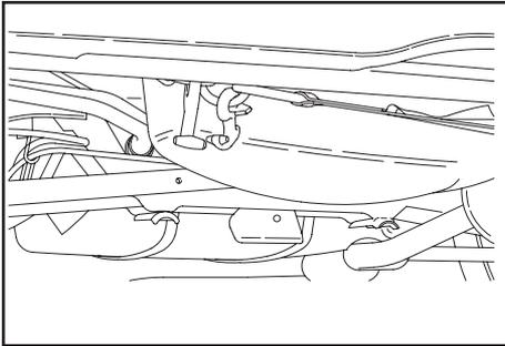
1. Using the RTJ hook cluster straps and ratchet spool mechanisms, insert the appropriate hook into the vehicle frame tie down hole or slot. **Refer to the AAA or vehicle manufacturer's towing manual for the correct attachment points.**
