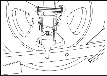
1. With the vehicle lifted just barely off the ground, attach the strap to the wheel restraints. Be sure the hook on the ratchet is securely seated in the wheel restraint.
