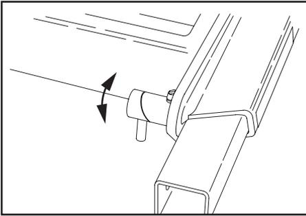
6. Take the L-Arms and slide them into the channels on the side of the grid. Make sure that they are resting snugly against the tires, with the L-Arms in close contact with the tires. Then reset the locking pin by turning the "Cam" handle back to the original position. The tires are now confined front and back.
