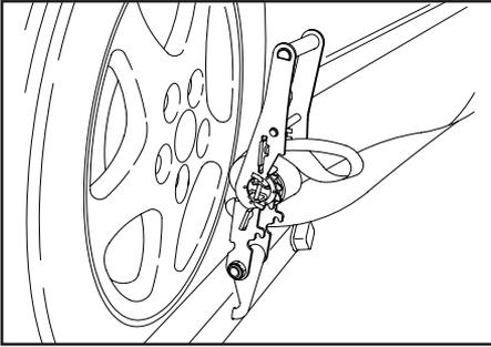
1. With the vehicle lifted just barely off the ground, attach the strap to the L-Arm. Be sure the hook on the ratchet is securely seated in the L-Arm.
