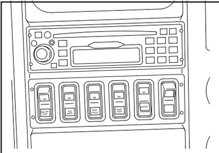
1. Turn on the body lights and any work lights, as necessary. (Switches are located on the switch panel in the dash).
