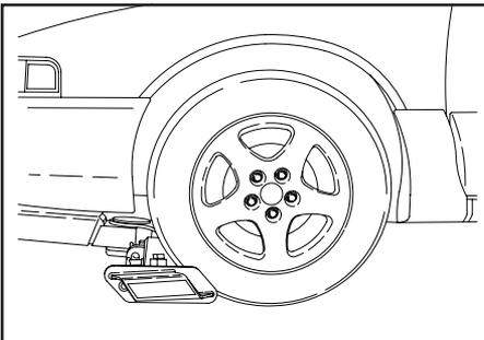
4. Extend the lift arm under the casualty vehicle. Make sure that all under carriage parts are cleared and that the front portion of the grid is in contact with both tires. Lower the grid fully to the ground.
