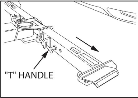
2. To set the grid width, loosen the "T" handles on the front of the grid arms and pull out. Be sure both grids are as close to the center of the boom as possible, and wide enough to allow the L-Arms to slide into their channels. Tighten the "T" handles to secure the grids.
