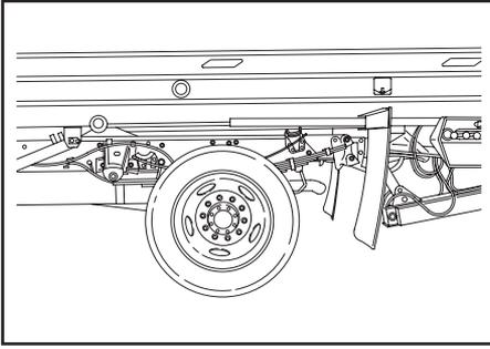
18. Remove the wheel chocks from the carrier's rear tires.
