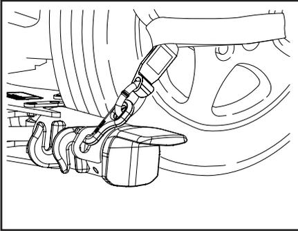
3. Place the hook of the strap assembly into a hole on the front side of the grid.
