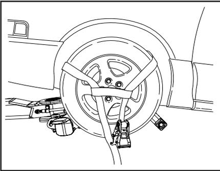
1. With the vehicle lifted just barely off the ground, insert the end of the strap through the sewn loop on the other end of the strap to form a loop. Put the loop over the tire as shown with the strap resting on the tire at the ten o'clock and two o'clock positions. Place the choker strap across the center of the tire..
