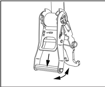
1. First set the spool into “free spool”. This is done by pulling the lock bar out and swinging the handle upward until it rests in the free spool notch and then simply pulling out the amount of strap required to fit over the tire.
