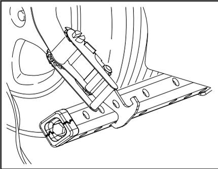
2. Place the hook of the ratchet assembly into a hole on the back side of the grid arm. Use the hole that is closest to the tire.
