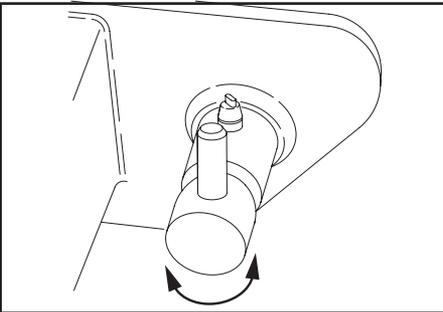
3. Retract the "Cam" handle locking pin on the grid by turning it 180°. It should remain in the open position.
