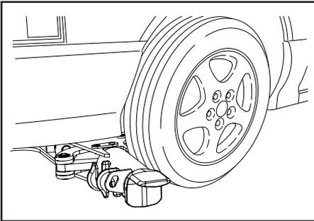
2. Extend the lift arm under the casualty vehicle being sure that all under carriage parts are cleared and that the front portion of the grid is in contact with both tires. Lower the grid fully to the ground. If using a remote hand controller, the underlift level stop assist system will stop the underlift travel at a preset position about 1-1/2" to 2" from the ground.
