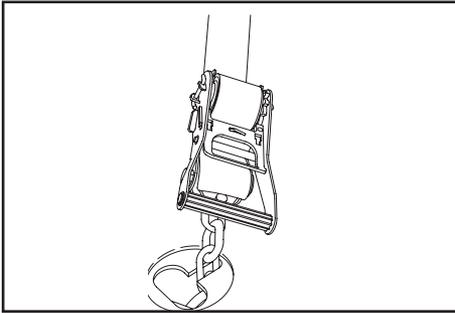
2. Insert the chain on the end of the ratchet into the keyslot in the deck. Adjust the chain so that it is as tight as possible. Using the ratchet, tighten the tie down strap.
