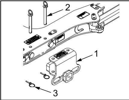
3. Place the reese hitch adapter bracket (1) onto the hydraulic grid crossbar.
