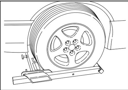
9. Load the vehicle onto the wheel lift. **(See Wheel Grid Operation, Sections 4.7, 4-8 and 4.9)**
