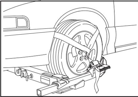
2. Set the ratchet spool in "free spool" position and pull the webbed strap out and form a loop which will wrap around the tire. Be sure the loop is over a minimum of 1/3 of the tire.
