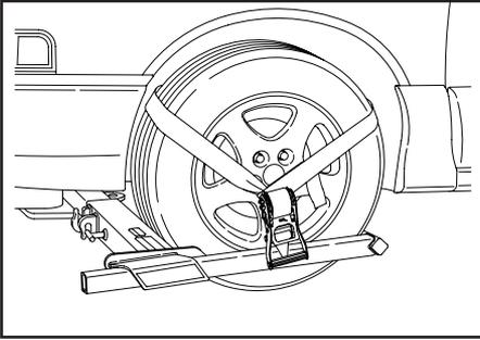
11. Install tie-down straps to secure the wheels in the grid. (See **Tie-Down Straps Installation, Sections 4.10, 4-11 and 4-12**)
