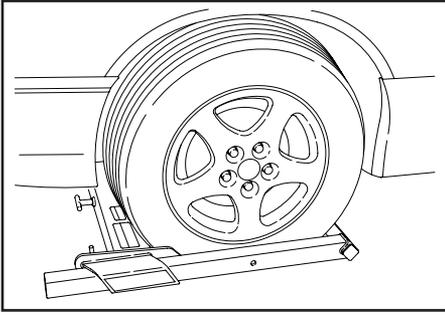
5. Visually inspect the tire to grid contact before proceeding.
