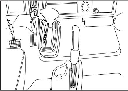
3. Place the carrier's transmission gear selector into Neutral or Park and set the parking brakes.
