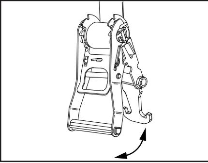
3. Now pull on the lock bar and move it downward until it engages the ratchet teeth on the take-up spool. By pushing and pulling the handle up and down, the strap will be wound onto the spool.
