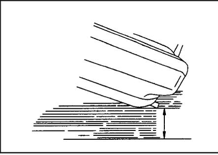
14. Make sure that the far end of the vehicle has enough ground clearance. It is possible to set the rear of a front lifted vehicle completely on the ground. Take irregular road surfaces into consideration. Make sure that there are no under body components of the vehicle in contact with the L-Arms or wheel grid device. Readjust if necessary.
