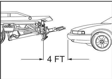
2. Position the rear of the carrier about 4 feet from the vehicle you intend to load. Make sure you are in line with the vehicle to tow.
