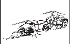
• Don't tow a vehicle on its front wheels if they are damaged.
