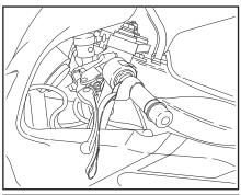
15. Tie the front of the motorcycle to the rear of the wrecker body. Attach the lasso style straps to each of the handle bars.
