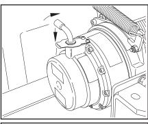
10. Re-engage the winch drive by pushing down on the spring steel latch plate and turning the handle 180°. Confirm winch engagement by jogging the winch control. Now slowly take up the slack in the wire rope.
