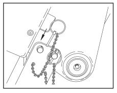
3. Secure the hitch pins with the linch pins.
