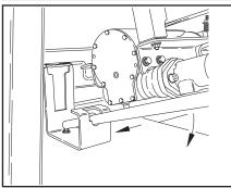
6. Afterloading the dollies, place the pry bar/jack bar back into the storage bracket by inserting the end of the bar with the ring around it thru the cutout in the front bracket. Allow the other end of the bar to rest on the rear bracket.
