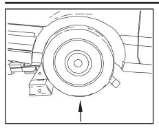
13. Lift the vehicle high enough to allow the tires to clear the ground. Make sure that the grid is not in contact with any engine or body components.
