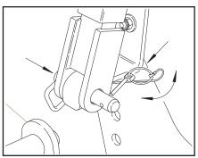
28. Connect the hold back bars to the tow sling storage brackets using the pins that you removed earlier.
