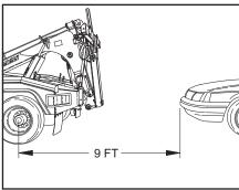
Position the truck within 9 ft. of the subject vehicle and as close to the direction of the tow as possible.
