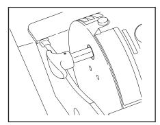
Reengage the winch "free-spool" by turning the handle back 90°.
