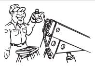
Lubricate and maintain both the wire rope and winch on regular intervals. (See maintenance charts.)
