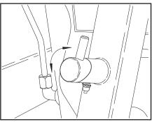
29. Rotate the "CAM" handles on the hold back bars 180° to the closed position.
