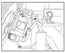
2. Open dolly the retaining latch by pulling the top toward you.
