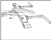
5. Completely retract the wheel grid for loading.
