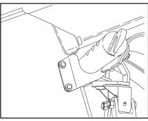
Lower the boom to allow the tow sling head to raise out of it holder on the back side of the boom.
