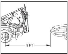
Position the truck within 9 ft. of the subject vehicle and as close to the direction of the pull as possible.
