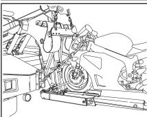
16. Place the hook on one end of the "front" strap to the loop of the lasso strap on the handle bars and place the hook on the other end to the rear of the wrecker body and tighten with the ratchet. Repeat for the other side.
