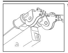
13. Now slowly retrieve the wire rope, carefully winding the wire rope onto the drum. Many operators take this opportunity to do a visual inspection. When you've finished rewinding the wire rope, be sure you don't overwind it. Always wear safety glasses and gloves when doing recovery work or handling the wire rope.
