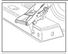
Place the hook of the ratchet into one of the holes on the front side of the grid. Again, try to use the hole that is closest to the tire.
