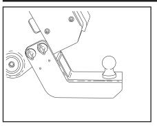
4. Install the desired towball to the towball hitch.
