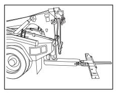
6. Unhook the wire rope cables from the top of the tow sling.
