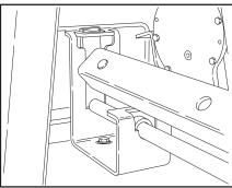
12. Allow the axle cross tube rails to hang from the bracket by the tab.
