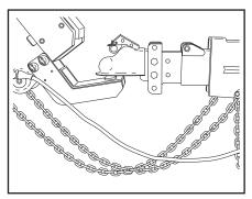
6. Connect the trailer lights and attach safety chains.
