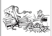
You should never make a lift or movement while close to or under the vehicle being lifted!
