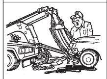
Never attach the chain hooks in such a way as to damage brake lines or other functional parts.
