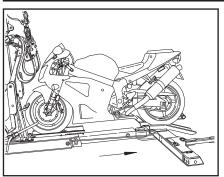
12. After securing the front tire, extend the wheel lift under the rear tire of the motorcycle raising the rear tire of the motorcycle onto the ramp.
