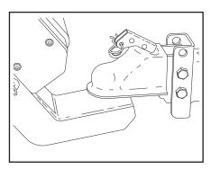
5. Position the ball coupler over the ball and lock into place.
