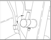
7. Rotate the "CAM" handles on the hold back bars 180° to the close position. Raise or lower the boom slightly until the cam locks on the tow sling hold bars snap into the closed position.
