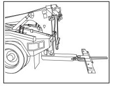
6. Unhook the wire rope cables from the top of the tow sling.
