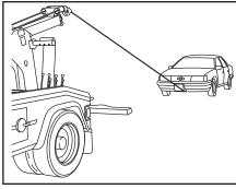
13. Once the work is in the desired position, apply the towed vehicles parking brake or use blocks or tie the work down if there is any question about stability. Slowly reduce the wire rope tension. After enough wire rope has been unwound, you may remove the hookup.
