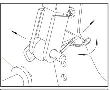
Remove the tow sling hold back bar retaining pins allowing the hold back bars to swing out of its retaining brackets on the sides of the boom.
