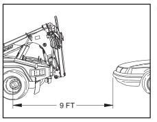
Confirm the truck's position in relation to the vehicle to be towed. Nine (9) feet is recommended. Reposition the MPL40 if necessary. Be sure the towed vehicle is not in gear or park. Keep the brake set.
