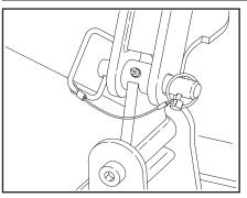
Connect the hold back bars to the tow sling lugs using the pins that you removed earlier.
