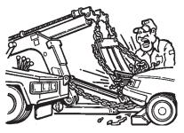
Be sure the chains and hooks are attached to frame members and not sheet metal.
