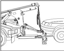
21. Retract the boom slowly drawing the vehicle forward until the stand offs are fully retracted and the "CAM" handles retract to the closed position for traveling.
