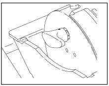
7. Disengage the winch "free-spool" by pulling out on the "T" handle and turning the handle 90°. The handle should remain in the "free-spool" position. Never turn this handle while the wire rope is under load! This allows the wire rope to be pulled directly off the drum to the work.
