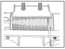
12. With the wire rope tight, slowly wind it in, observing both the work and the drum. Be sure the wire rope strands do not cross wrap or criss-cross on the drum. Observe the path the work must travel for snags or obstructions which could stall the movement and overload the wire rope.
