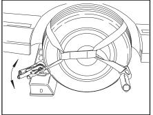
4. Take up the slack in the strap by ratcheting the takeup spool arm. Continue until the tires show some compression. Notice that the strap in the ratchet is pulling down and forward on the loop over the tire.
