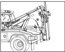
30. Retract the wrecker boom, snug up the wire rope(s) and fold up the underlift.
