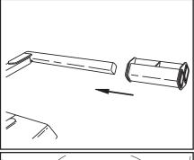
1. Slide the back side of the wheel spacer over the wheel grid arm.
