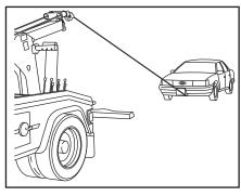
12.Once the work is in the desired position, apply the towed vehicles parking brake or use blocks or tie the work down if there is any question about stability. Slowly reduce the wire rope tension. After enough wire rope has been unwound, you may remove the hookup.
