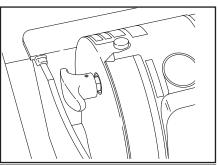
Jog the winch control until the handle retracts into the engaged position. Now slowly take up the slack in the wire rope.
