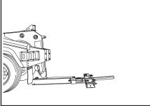
4. Unfold the under lift boom.
