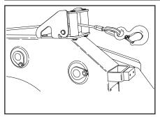
Pull the wire rope off of the winch spool and route it through the roller guide. Unwind enough wire rope to make the hook-up being sure that a minimum of at least five (5) wraps of wire rope remains on the drums.
