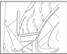
10. Check front tire for fit with the upper and lower tire stops. When the motorcycle is rocked side to side the front tire should feel solid in the tire stops and centered in the trough. If the front tire is not clamped in the stops, back the motorcycle off and readjust the stops as necessary.
