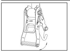
To release the ratchet, simply pull on the locking bar, disengaging the teeth and raise the handle to the "free spool" position.
