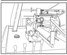
The axle cross tube rails need to be stored with the wheel ramp plates turned in and up.
