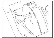
8. Reengage the winch "free-spool" by turning the handle back 90°.
