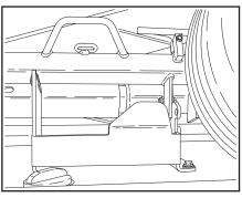
14. The tab on the storage bracket should be placed through the dolly pocket of the dolly wheel assembly.
