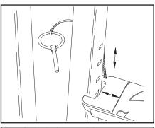
Adjust the upper and lower tire stops so that they will contact and restrain the front tire when loaded.
