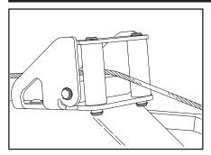
12. Now slowly retrieve the wire rope, carefully winding the wire rope onto the drum. Many operators take this opportunity to do a visual inspection. When you've finished rewinding the wire rope, be sure you don't overwind it. Always wear safety glasses and gloves when doing recovery work or handling the wire rope.
