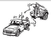
After rigging wire ropes, don't begin pulling without rechecking connections. Make sure that all wire ropes and snatch blocks are securely attached and cannot accidently pull loose.
