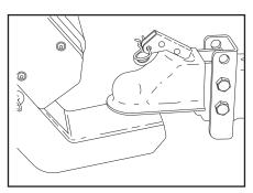
5. Position the ball coupler over the ball and lock into place.
