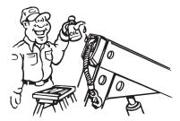
Lubricate and maintain both the wire rope and winch on regular intervals. (See maintenance charts.)
