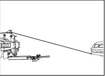
10. With the wire rope tight, slowly wind it in, observing both the work and the drum. Be sure the wire rope strands do not cross wrap or criss-cross on the drum. Observe the path the work must travel for snags or obstructions which could stall the movement and overload the wire rope.
