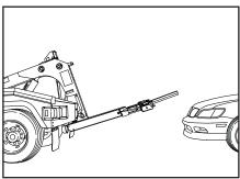
7. Next, lower the underlift using the underlift down function on the hand controller. The underlift level stop assist system will stop the underlift travel at a preset position about 1-1/2" to 2" from the ground.
