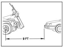
Confirm the truck's position in relation to the vehicle to be towed. Nine (9) feet is recommended. Reposition the MPL if necessary. Be sure the towed vehicle is not in gear or park. Keep the brake set.
