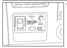
4. Engage the Power-Take-Off (PTO) or Clutch Pump and the hand controller using the "Control" switch in the switch panel. Most trucks will automatically throttle up when the parking brake is set and the transmission is park or neutral. NEVER TRAVEL WITH THE POWER-TAKE-OFF or CLUTCH PUMP CONTROL ENGAGED. This could result in damage to the PTO or Clutch Pump unit and the truck transmission.
