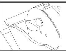
5. Disengage the winch "free-spool" by pulling out on the "T" handle and turning the handle 90°. The handle should remain in the "free-spool" position. Never turn this handle while the wire rope is under load! This allows the wire rope to be pulled directly off the drum to the work.
