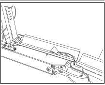
Attach the lower trough and vertical stop into the mounting bracket at the front of the boom with the pin and retaining pin.
