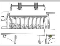
11. Once the work is in the desired position, apply the towed vehicles parking brake or use blocks or tie the work down if there is any question about stability. Slowly reduce the wire rope tension. After enough wire rope has been unwound, you may remove the hookup.
