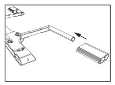
Slide the back side of the wheel spacer over the wheel grid arm.
