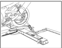
13. Tie down the rear of the motorcycle. Place the hook on one end of the "rear" strap into the hole on the front side of the grid. Place the other hook onto the motorcycle and tighten. Repeat for the other side.
