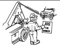
Jog the winch control lever to be sure of complete engagement of the clutch gears before making a lift or pull.
