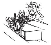
To avoid birdnesting and premature failure of the wire rope, always keep tension on the wire rope when unwinding.
