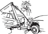
Never make a lift or pull with the wire rope attached to light gauge or sheet metal parts; use the frame or major structural members.
