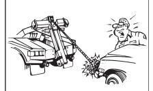
Never wrap the wire rope around frames or cross members. Use chains and hook the wire rope to the chains.
