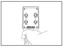
Using the hand controller, unfold the underlift using the tilt down function. The underlift level stop assist system will stop the underlift travel at a preset position.
