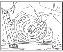
Push the motorcycle up the ramp until the front wheel is resting in and against the tire stops in the front brackets.
