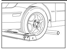
13. Lift the vehicle high enough to allow the tires to clear the ground. Make sure that the grid is not in contact with any engine or body components.
