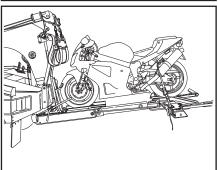
Raise the underlift boom to the desired towing height.
