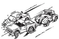
Don't tow a vehicle on its front wheels unless the steering wheel is secured with the front wheels straight ahead.
