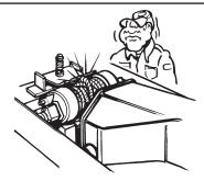
Never allow the wire rope to cross wrap (criss-cross) on the winch drum. Crushing of the wire rope can cause wire rope failure.
