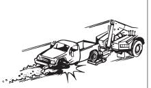
Don't tow a vehicle on its front wheels if they are damaged.
