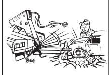
You should never make a lift or movement while close to or under the vehicle being lifted!
