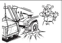
Avoid using the boom raise or boom up control to lift a load. This causes undue stress and weight loading on the rear axle.
