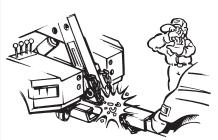
Check that the chain does not become over tensioned when raising the towed vehicle to the towing position or during the towing operation.
