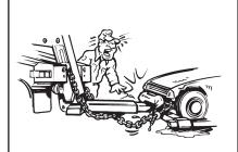
Never attach the chain hooks in such a way as to damage brake lines or other functional parts.
