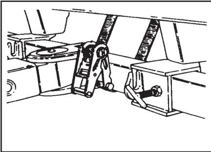
8. Secure the vehicle to the wheel grid crossbar with straps and ratchets.
