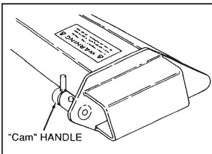
4. Retract the “Cam” handle locking pin on the grid by turning it a half turn. It should remain in the open position.
