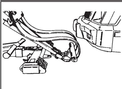
4. Lower the tow sling on the skid plate so that it will easily clear the bottom of the vehicle.
