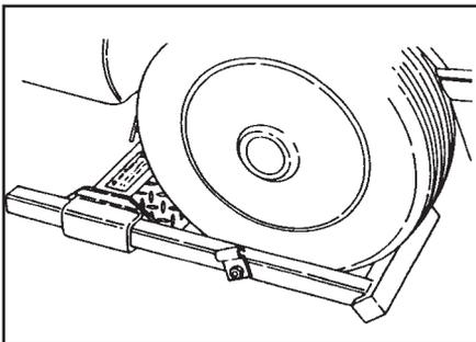
6. Take the “L” arms and slide them into the channels on the side of the grid. Insure that they are resting snugly against the tires. With the “L” arms in close contact with the tires, retract the locking pin by turning the “Cam” handle back to the original position. **Be sure that the pin seats in one of the holes.** The tires are now constrained front and back.
