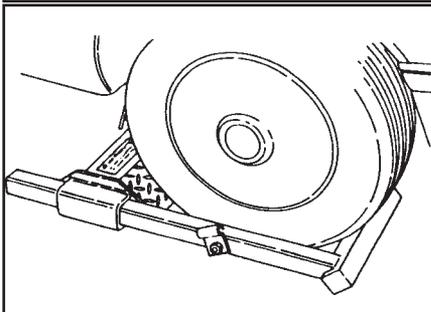
10. Secure the grid arm around the towed vehicle's tires following the instructions given for your particular grid option.
