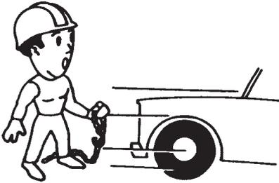
11. Complete the lift or pull being sure the work is placed in a stable location where it won't slip or roll. Use blocks or tie the work down if there is any question about the stability after the wire rope/cables and chains are removed.
