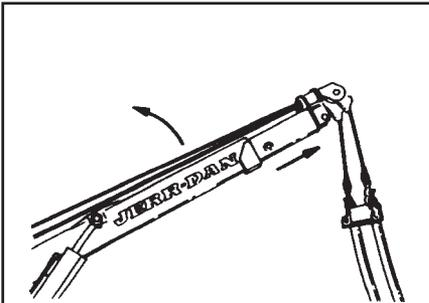
1. Raise the wrecker boom to approximately 45° and telescope out to allow for working clearance.
