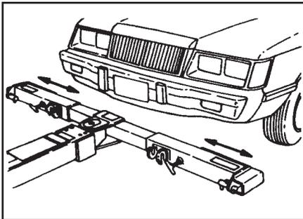
7. Set the grid width as required for the vehicle to be towed. Be sure both grids are as close to the center of the boom as possible. (See your particular grid option instructions.)
