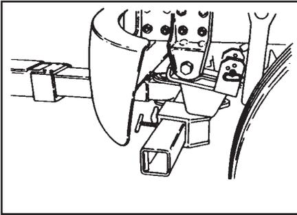
6. Move the lift attachments under the vehicle so that they are in the proper position for lifting. **At the same time make sure you are not attaching the lift attachments to any steering components.**
