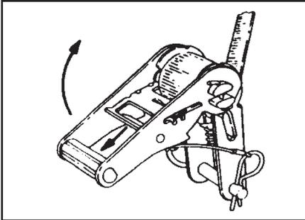
1. First the spool must be set into "free spool". This is done by pulling the lock bar out and swinging the handle upward until it rests in the free spool notch and then simply pulling out the amount of strap required to fit over the tire.
