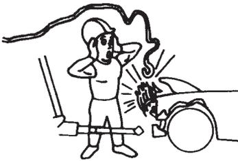
5. Attach the chain sling, hook or wire rope/cable hook securely to the work. Be sure of this hook up; you don't want it breaking loose during the pull. (See the safety sections earlier in the manual).
