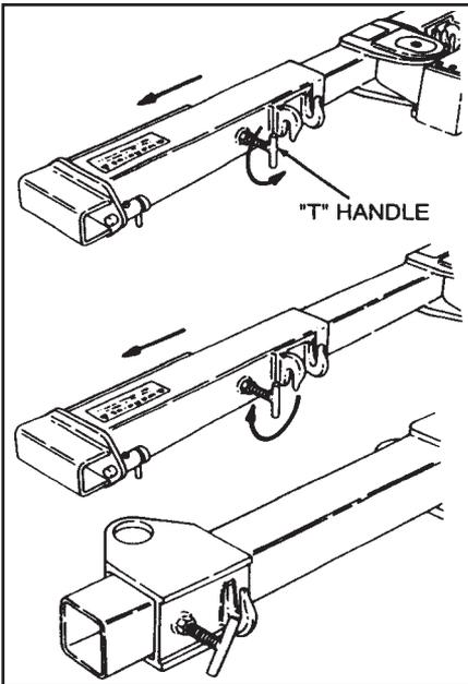
1. First, you will need to remove the wheel lift grids and install the lift attachment receivers.
