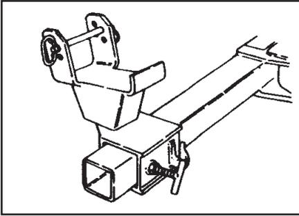
5. Now, choose the lift attachments that are best suited to your need and insert them into the receivers that you just put onto the crossbar. (Frame forks are for lifting by axles and frame crossmembers, spring hanger attachments are for lifting by leaf springs).
