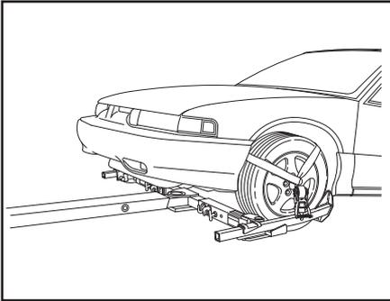
4. Raise the wheel grid to the towing position. **RE-TIGHTEN THE RATCHET PERIODICALLY AS THE TIRE SETTLES IN GRID FROM TOWING.**
