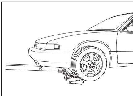
4. Extend the lift arm under the casualty vehicle. Make sure that all under carriage parts are cleared and that the front portion of the grid is in contact with both tires. Lower the grid fully to the ground. **There is no reason for the operator to get under the casualty vehicle.**
