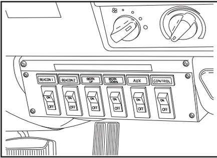
1. Turn on the safety and work lights. (Switches located on the dash panel).
