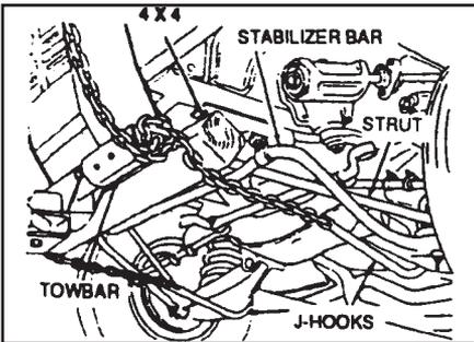
5. Maneuver the sling under the vehicle to be towed, far enough under so the vehicle will ride on the rubber belts.
