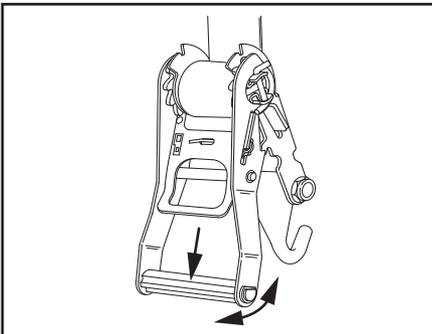
1. First set the spool into "free spool". This is done by pulling the lock bar out and swinging the handle upward until it rests in the free spool notch and then simply pulling out the amount of strap required to fit over the tire.
