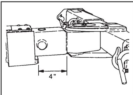
17. Power retract the grid boom until the towed vehicle is about 3 to 4 feet from the back of the truck. Leave enough room to maneuver around corners without corner binding or causing contact between the two (2) vehicles. **Be sure that the boom is extended at least 4" to ensure unobstructed crossbar pivoting.**
