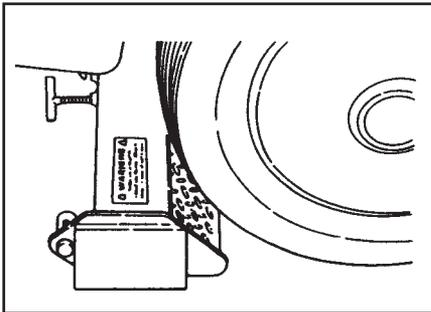
8. Extend the lift arm under the vehicle being sure that all under carriage parts are cleared and that the front portion of the grid is in contact with both tires. Lower the grid fully to the ground. **There is no reason for the operator to get under the vehicle.**
