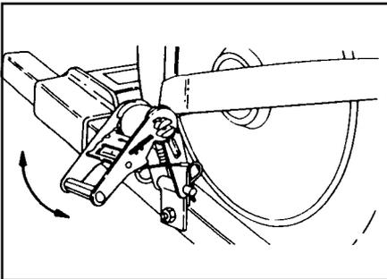
2. Set the ratchet spool in "free spool" position and pull the webbed strap out and form a loop which will wrap around the tire. Be sure the loop is over approximately 1/3 of the tire.
