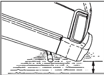
16. Raise the vehicle into the final towing position observing the far end for sufficient ground clearance. It is possible to set the rear of a front lifted vehicle completely onto the ground, causing damage. Take irregular roadsurfaces into consideration. Observe the lift function from the side and away from both vehicles if possible.
