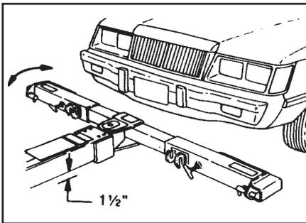
6. Lower the lift arm to about 1-1/2" from the ground and swing the cross bar parallel to the tires.
