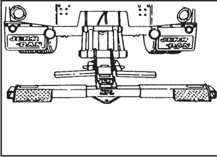
3. Set the brakes on your Jerr-Dan unit. If the pull will be a heavy one you may also use the controls to set the grid boom down on the ground giving the truck more traction and resistance to slippage. The use of scotch blocks is also recommended.
