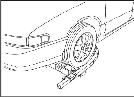
6. Take the wheel restraints and place them into their receivers on the side of the grid. The restraints should be placed in a position as close as possible to fit the tires. **Be sure that the holes in the bottom of the restraints lock over the retaining pin on the receivers.**
