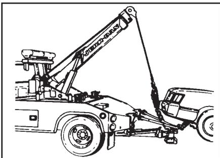
9. Raise the vehicle using the wrecker boom winch. (Read the safety and operating instructions for the boom and winch beforehand.) The vehicle should be raised until the wheels are a minimum of ten inches off the ground. Observe the opposite end of the vehicle for ground clearance.
