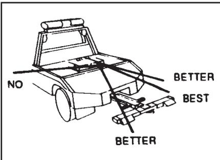
2. Position and align the truck to obtain as direct a pull as possible. Straight line pulls are the best and most efficient.
