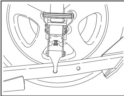
1. With the vehicle lifted just barely off the ground, attach the strap to the wheel restraints. Be sure the hook on the ratchet is securely seated in the wheel restraint.
