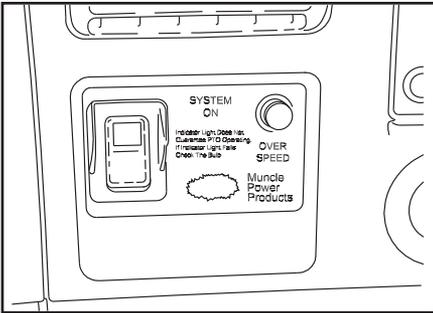
4. Engage the Power-Take-Off (PTO) or Clutch Pump and the hand controller using the "Control" switch in the switch panel. Most trucks will automatically throttle up when the parking brake is set and the transmission is in park or neutral. **NEVER TRAVEL WITH THE POWER-TAKE-OFF or CLUTCH PUMP CONTROL ENGAGED.** This could result in damage to the PTO or Clutch Pump unit and the truck transmission.
