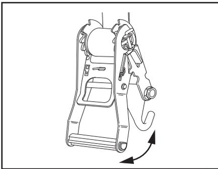
3. To release the ratchet, simply pull on the locking bar, disengaging the teeth and raise the handle to the "free spool" position.
