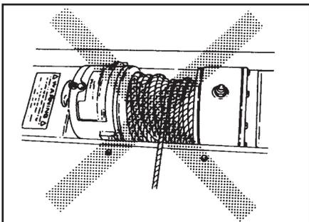
7. With the wire rope/cable tight, slowly bring it in, observing both the work and the cable drum. Be sure that the wire rope /cable does not cross wrap or criss-cross on the drum. Observe the path the work must travel for snags or obstructions which could stall the work movement and overload the wire rope/cable.
