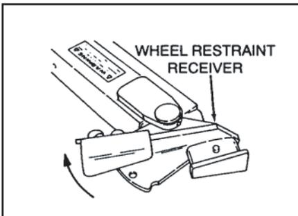
3. Pivot the wheel restraint receivers on the end of the grid arms outward by lifting up on the receiver. Rotate the "Cam" handles on the receivers 180° to the open position for easier placement of the restraint into the receiver.
