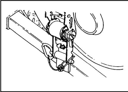
1. With the vehicle lifted just barely off the ground, attach the strap to the wheel grid. Be sure the ratchet pin is secured with the hairpin cotter pin.
