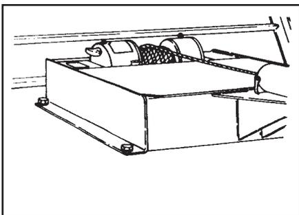
9. Now slowly retrieve the wire rope/cable, winding it back onto the drum. Many operators take this opportunity to do a visual inspection. When you've finished respooling the wire rope/cable, be sure you don't overwind it. Always wear safety glasses and gloves when doing recovery work or handling the winch wire rope/cable.
