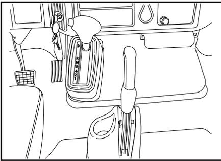
3. Set the truck's parking brakes and put the transmission in park or neutral.
