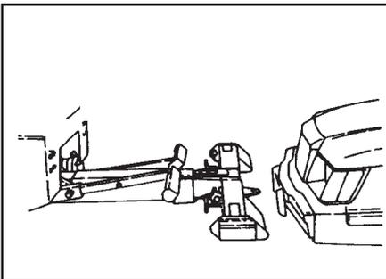
5. Confirm the truck's position in relation to the vehicle to be towed. Three (3) to four (4) feet is recommended. Reposition the HPL if necessary. **Be sure the towed vehicle is not in gear or park. Keep the brake set.**
