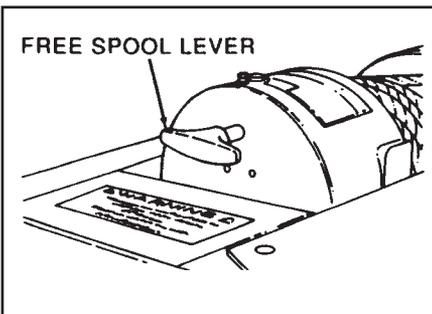
6. Re-engage the winch drive by turning the handle back 90°. It should retract cleanly. Jog the winch control lever to confirm engagement. Using the controls, slowly take up any slack in the wire rope/cable.
