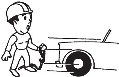
11. Complete the lift or pull being sure the work is placed in a stable location where it won't slip or roll. Use blocks or tie the work down if there is any question about the stability after the wire rope/cables and chains are removed.
