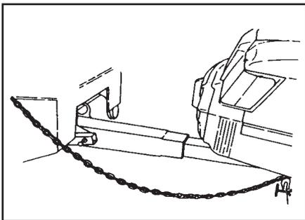
18. Be sure to maintain sufficient clearances with the bottom of the towed vehicle.
