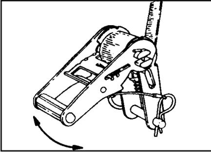
3. To release the ratchet, simply pull on the locking bar, disengaging the teeth and raise the handle to the "free spool" position.
