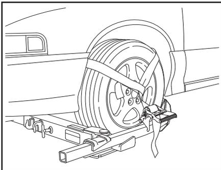
2. Set the ratchet spool in "free spool" position and pull the webbed strap out and form a loop which will wrap around the tire. Be sure the loop is over a minimum of 1/3 of the tire.
