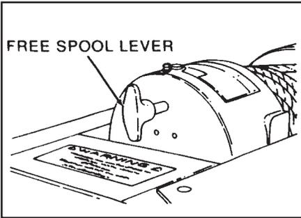
4. Release the free spooling lever on the winch by pulling and turning the handle 90°. **Never pull this while the wire rope/cable is under load!** This allows the wire rope/cable to be pulled directly off the drum to the work. Return to the wire rope/cable drum and be sure that at least five (5) wraps of cable remain on the drum.
