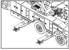
2. Using the controls, extend the outriggers to the full extended position.
