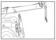
Manually, "free-spool" enough wire rope to make the hook-up being sure that a minimum of five (5) wraps remains on the cable drums.
