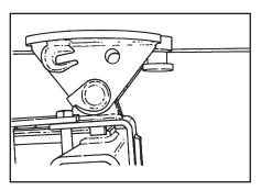
6. Extend the underlift boom and 5th wheel attachment up to the king pin of the casualty vehicle.
