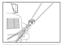
13. Activate the winch free-spool at the controls to re-engage both wrecker boom winches. Slowly take up the slack in the wire ropes. Inspect the hook-up points for slippage before continuing the lift or pull. Control each winch to ensure wire ropes are stressed evenly. As the wire rope is retrieved, be sure it doesn't crisscross on the spool.
