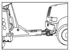
7. With the casualty vehicle in neutral and the parking brake released, the underlift can be raised, lowered, extended or retracted. All of these movements are hydraulically controlled.
