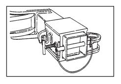
9. Attach the lift receivers to the crossbar by sliding them over the ends of the crossbar. The lift receivers are found in the body tool compartment. Install the retaining pin into the end of the crossbar and secure with the safety pin. Refer to VARIOUS POSITIONS FOR LIFT RECEIVER USE Section 4.2.
