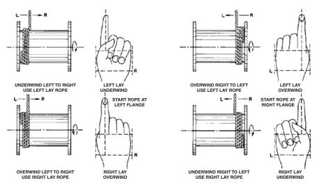
A simple method of determining how a wire rope should be started on a drum is shown above. The observer stands behind the drum, with the rope coming towards him. Using the right hand for right-lay wire rope, and the left hand for left lay wire rope, the clenched fist denotes the drum, the extended index finger the oncoming rope.
