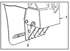
3. Line up holes and insert spade pin (2) and retaining pin (1).
