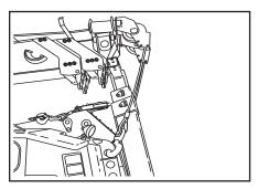
Unhook the wire ropes from their stored position. Moving the wrecker boom with the wire ropes hooked can result in damage to both the wire ropes and the boom.
