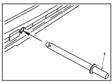
Remove the outrigger pins from the storages compartments. Install the pins (1) into the inner sections of the outrigger and secure with the retaining pins (2). (Three section outriggers only).
