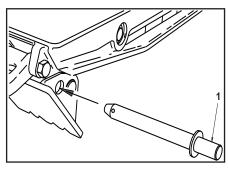
Line up holes and insert spade pin (1) and secure with the retaining pin (2).
