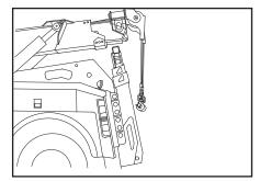
Position the boom head by using the boom up, down, in, out and slew left and right levers as necessary.
