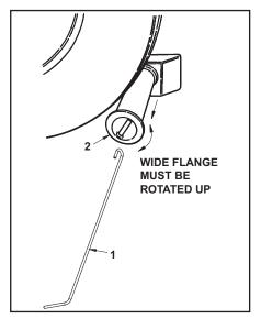
9. Using the pulling tool (1), extend the round tube (2) to capture the back of the tire. After extending the tube beyond the edge of the tire, make sure that the wide flanged edge of the tube is rotated up to prevent the tire from sliding off the end of the tube.
