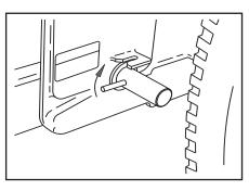
7. Install the pins into the outer sections of the outriggers.
