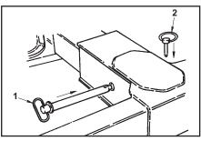
2. Install the retaining pin (1) from the back side of the crossbar through the grid and crossbar and secure with the pin (2).
