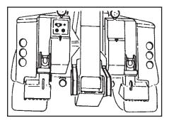
Position the recovery vehicle as close as possible to the casualty vehicle. Set the parking brakes, place the transmission in neutral and chock the wheels.
