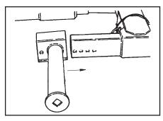
6. Slide the arm weldment over the end of the grid and adjust to the desired position for loading.
