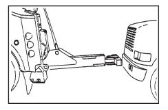
The recovery vehicle's position should be approximately nine (9) feet from the casualty vehicle. Reposition the recovery vehicle if necessary.
